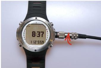
9.1.1 Attach the plug, red dots aligned, and turn the plug clockwise.
