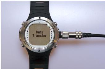
9.2.1 The dive computer (DC) will automatically switch into the transfer mode.
