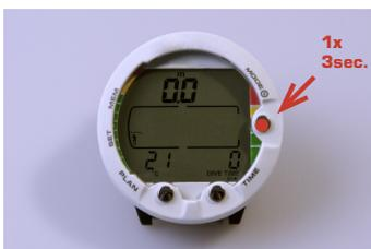
9.3.2 Switch on the dive computer (DC) and press the **mode** button for 3 seconds.
