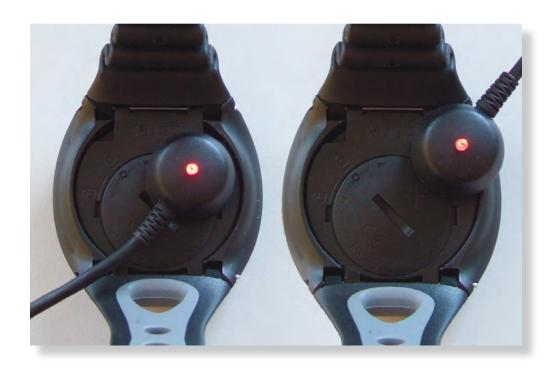
2.2 and connect the interface to your diving computer. The direction does not matter. The interface recognises the direction automatically and starts to illuminate red.
