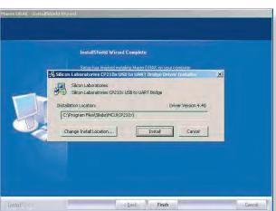
1.2 The USB driver for the interface is installed at this point. Confirm the installation path by clicking on "install".
