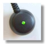
3.2 The interface has been recognised by the computer and a green LED is lit.
