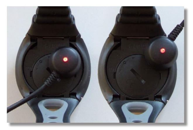
5.0 With a smartinterface the direction you choose to connect it with your dive computer doesn't matter. When conntected, the LED will shine red.
